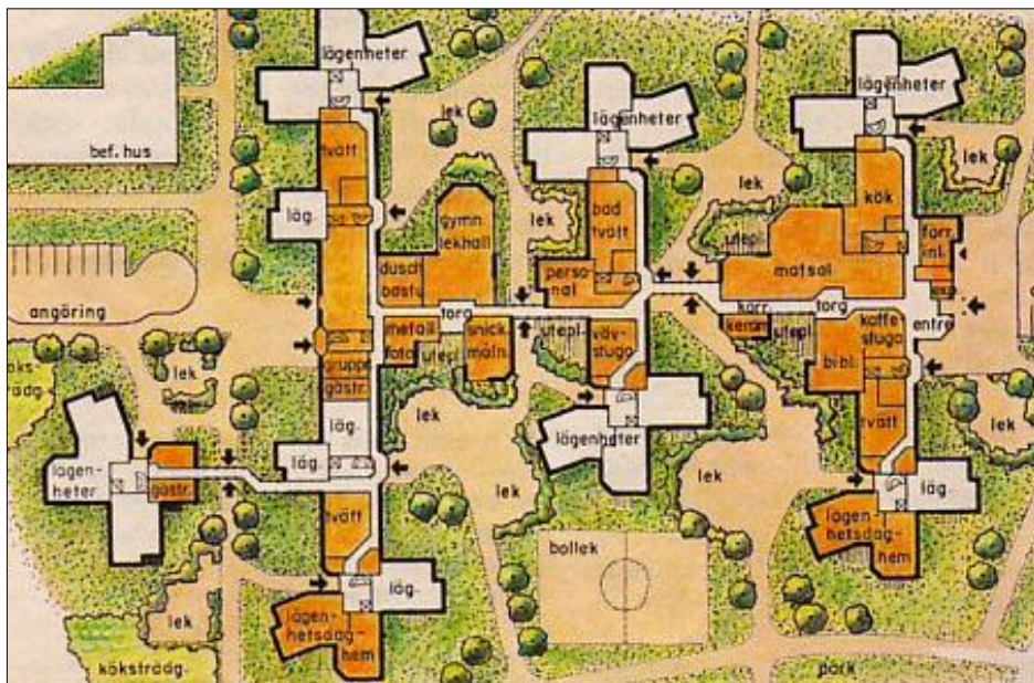
Fig 5. Plan of the ground floor of the cohousing Stolplyckan in Linköping, with 184 apartments. By abstaining from 10% of private apartment space the residents get access to 26 communal facilities, comprising altogether 2000 sqm.
